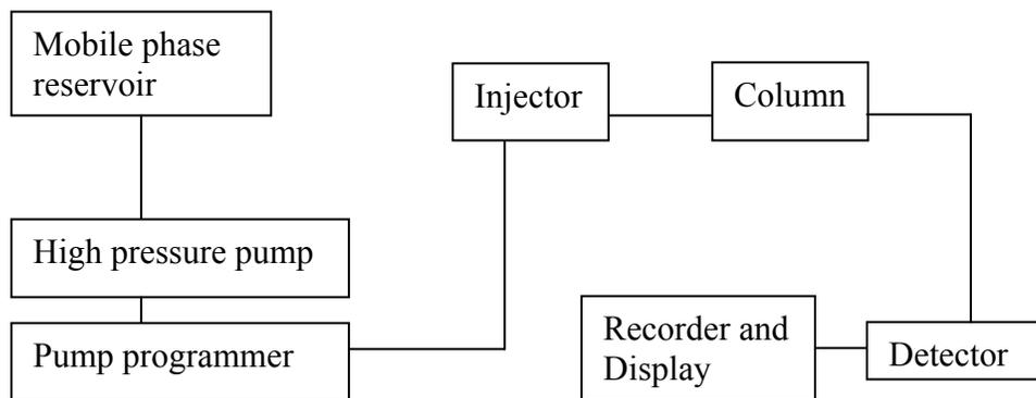
Figure 3. Schematic Diagram of the HPLC System
