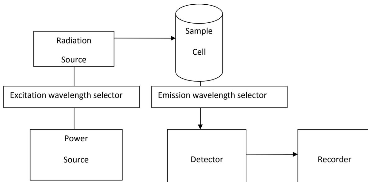
Figure 7: Schematic Diagram of the instrumental setup of a fluorometer
