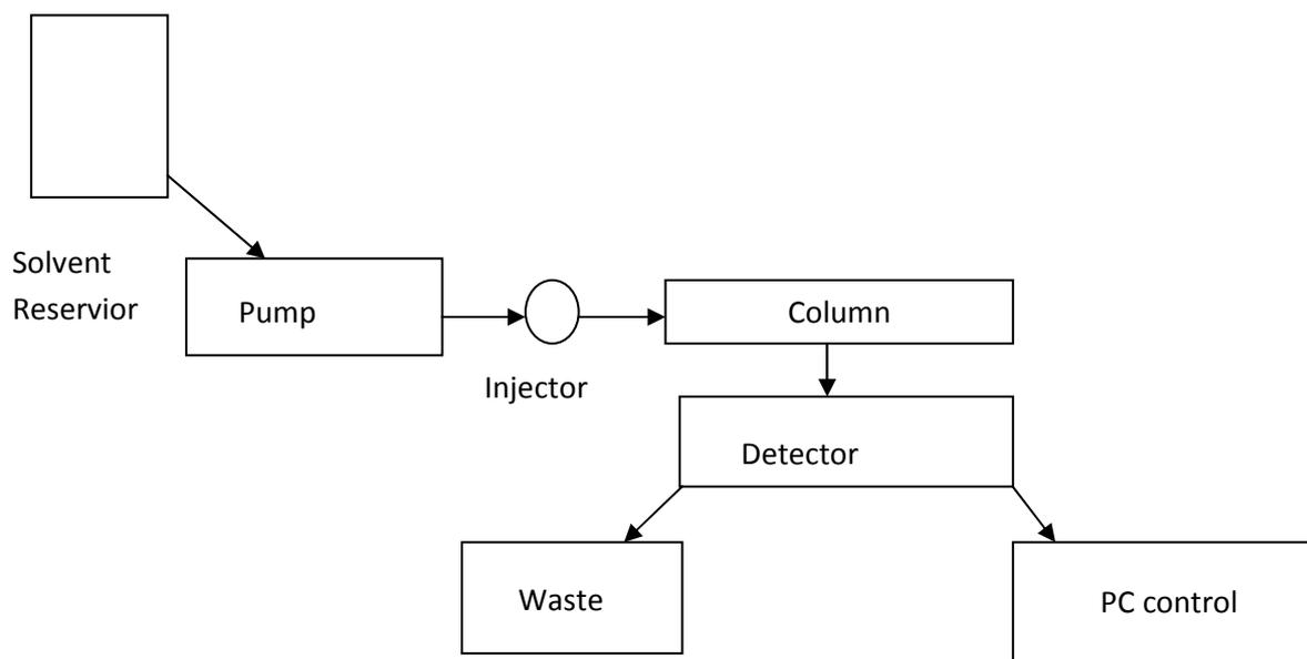
Figure 5: Schematic representation of high performance liquid chromatography
