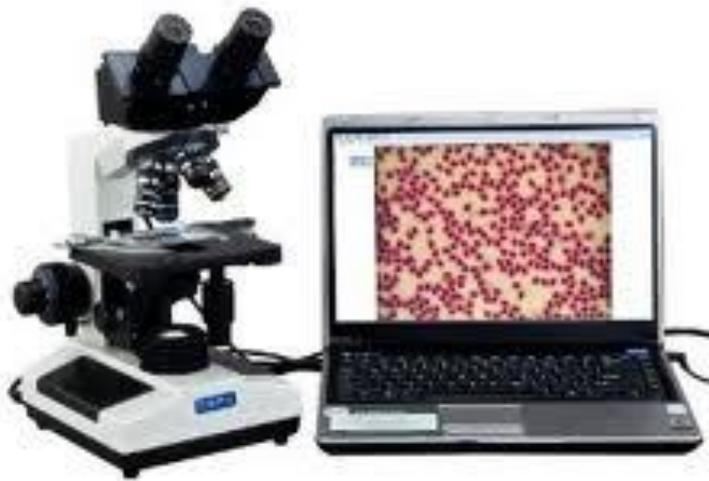
Figure 6: Using a digital camera microscope (manufactured by Nikonci, Japan), pictures were taken at 10X and 40X magnification for analysis.
