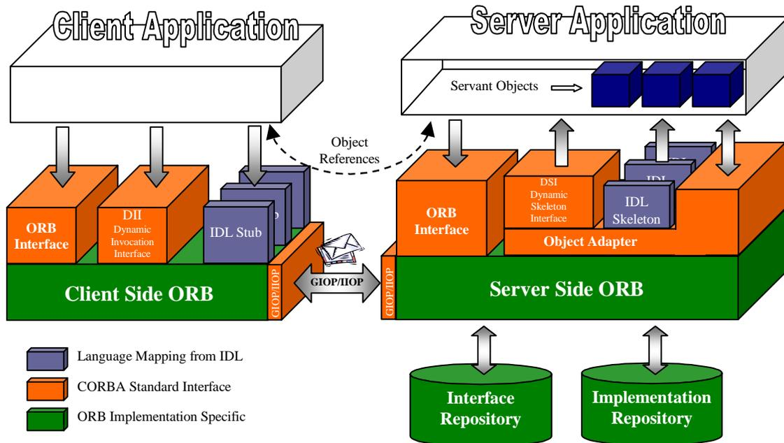
Figure 3 The Common Object Request Broker Architecture (CORBA)
