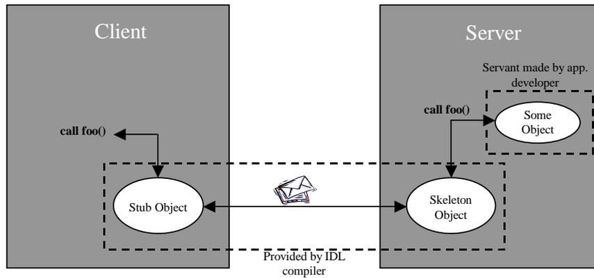
Figure 2 Relationship between Stub, Skeleton, and Servant
