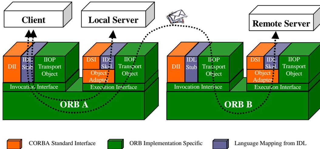
Figure 7 Method Invocation with the MICO ORB
