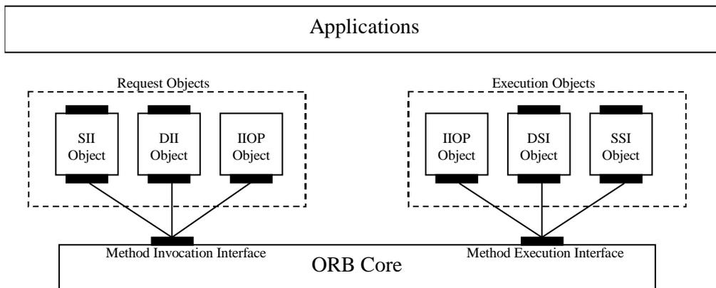
Figure 6 MICO ORB Design Model; adapted from [5]
