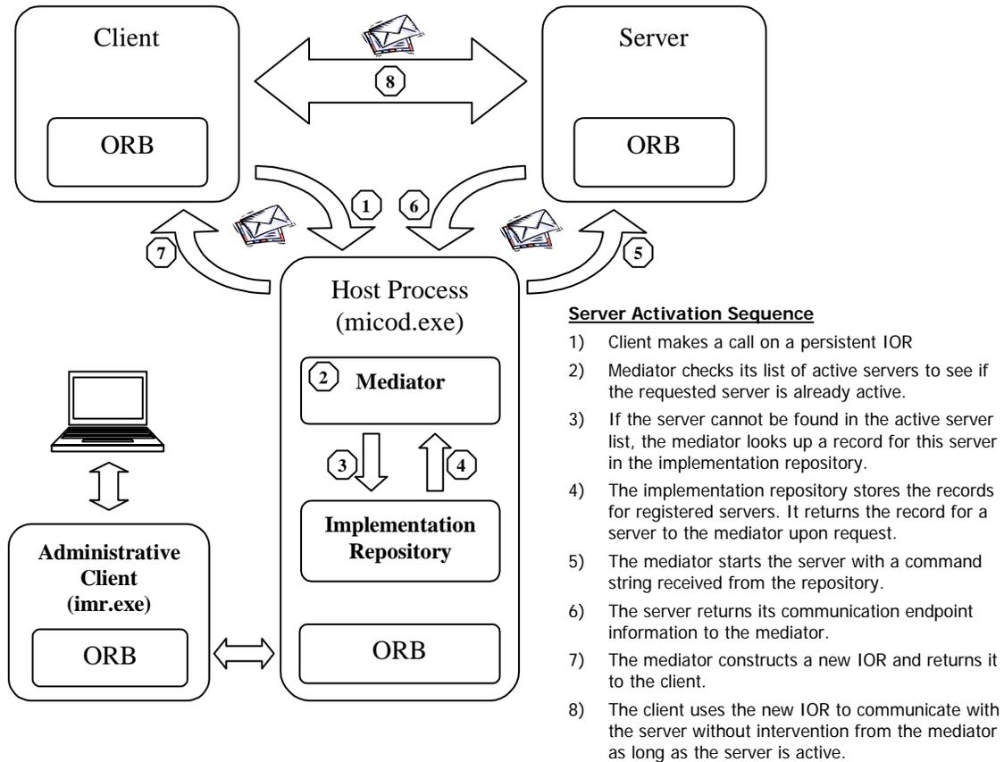
Figure 8 Structure of The MICO Runtime Service
