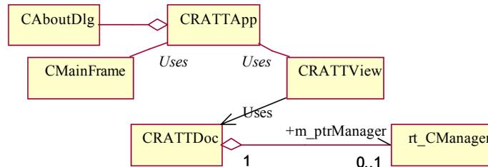
**Figure 5.2: Class Diagram For User Interface Module**
