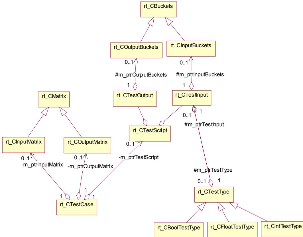
**Figure 5.3: Class Diagram For Data Storage Module**
