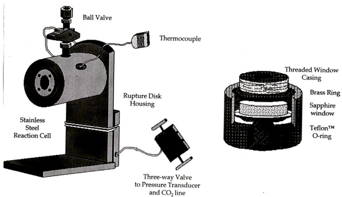
Figure 18. Structure of the constant volume cell
