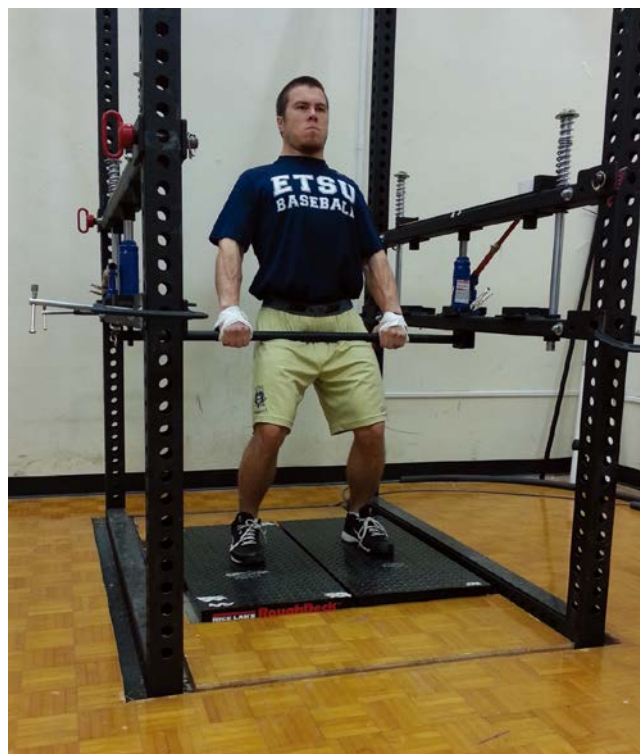
Figure 3 Photograph of isometric mid-thigh pull positioning on dual force plates.
