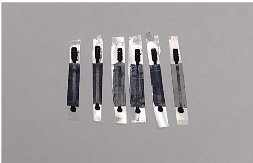
Figure 2. Sample electrodes fabricated from commercially available graphite ink and nitrogen-doped. The lower circular end of the electrodes denotes the working portion of the electrodes while connections to electrochemical systems are done at the other end.
