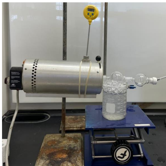
Figure 12. Apparatus for bulb-to-bulb vacuum distillation
