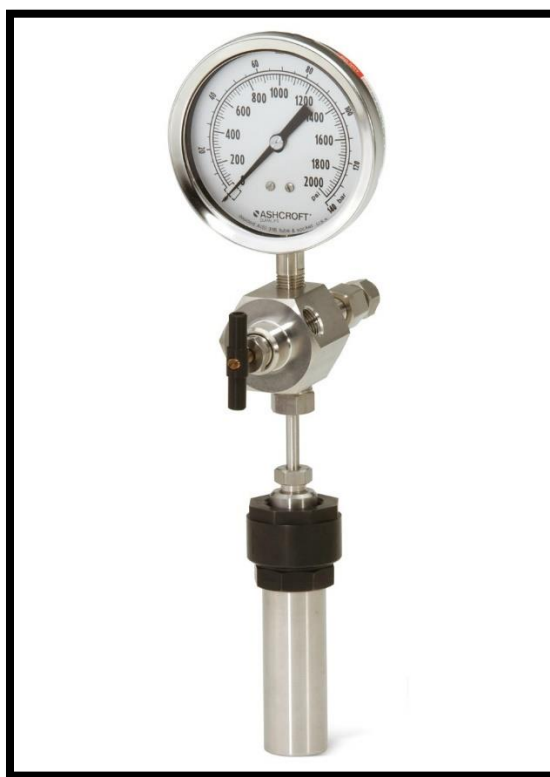
Figure 24. Parr 45 mL 4700 pressure vessel with 4310A gage block assembly. Used with permission. 47
