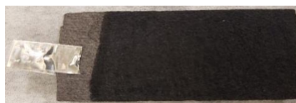
Figure 8. The film of hydrogen bronze after 7200 seconds of electrodeposition on the C-paper
