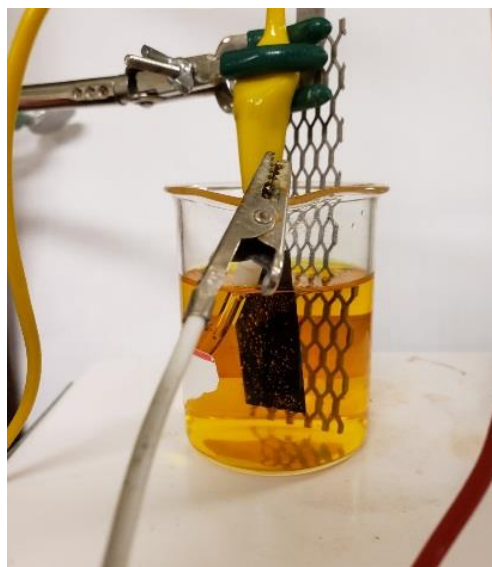
Figure 4. A photo of electrodeposition experiment
