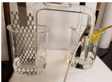
Figure 5. The employed electrochemical cell for the reduction trial of CO 2 in the lab
