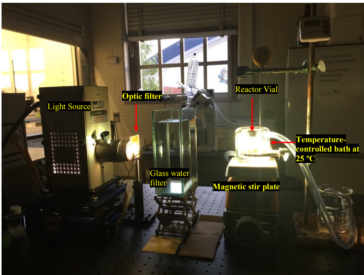
Figure 11. A picture shows the actual experimental components setup for photocatalysis reaction
