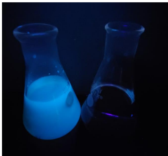
Figure 15. CDs solution ( 0.1 \text{ mg mL}^{-1} ) of sample B (left) and water (right) when view under a 4-Watt, 254/365 nm UVGL-15 Compact UV lamp.
