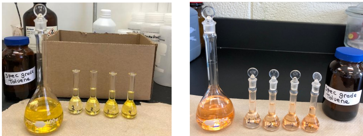
Figure 2.7. Different concentrations of ZnDPY (left) and ZnIDPY (right) complexes in toluene spectrophotometric grade for measuring the extinction coefficient
