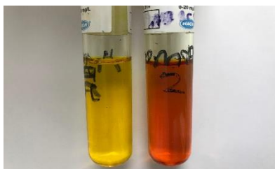
Figure 12. Color change before and after DNS method
