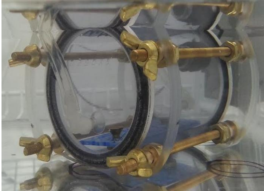
Figure 1. A partially submerged custom 90mL respirometer
