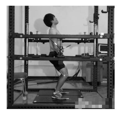
Figure 4.1 The isometric mid-thigh pull (IMTP) testing apparatus
