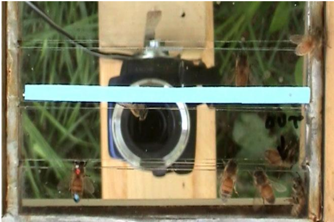
Fig. 1. Frame capture showing the entryway (from a camera mounted above it) to the observation hive from trial 2. Foragers were required to transit between two glass panes in order to enter or exit the hive. Seen in this frame is one individually marked forager (lower left, with white, red and blue paint dots; WRB) and several unmarked foragers. The hive entrance is at the top side of the entryway. A horizontal blue strip is positioned on the upper surface of the glass. A second video camera, pointing upwards, is positioned below the glass to record the identities of bees traversing the entryway upside-down.
