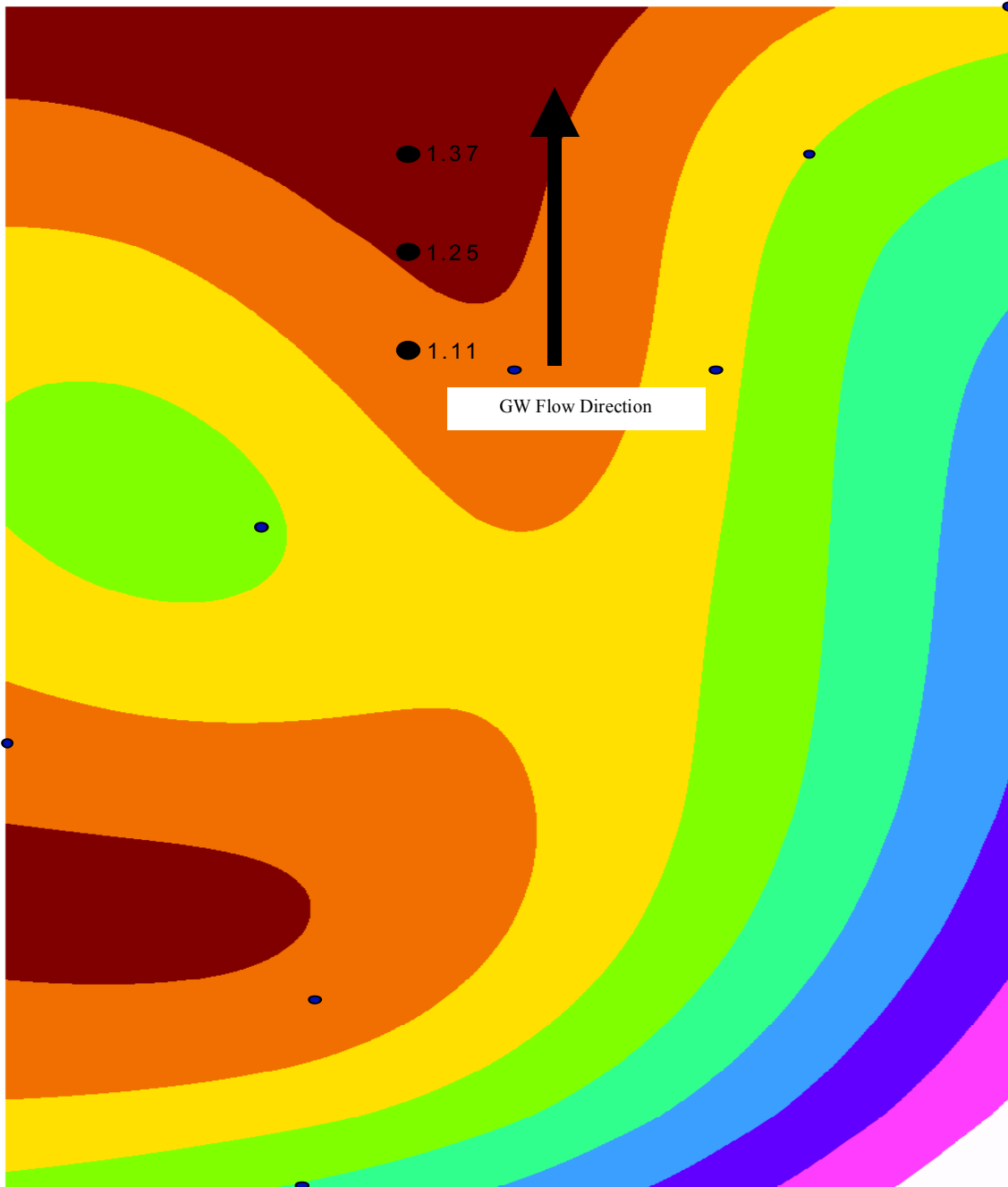
Figure 15 Interpolated 2D Map of Manganese Concentrations at Site N at T1 (<4 Weeks Post-ISCO)
