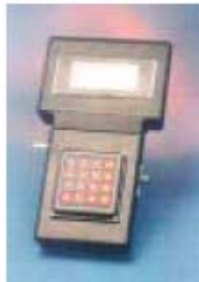
Figure 17. Standing Wave Reflectometer (Pappas, 2001).
