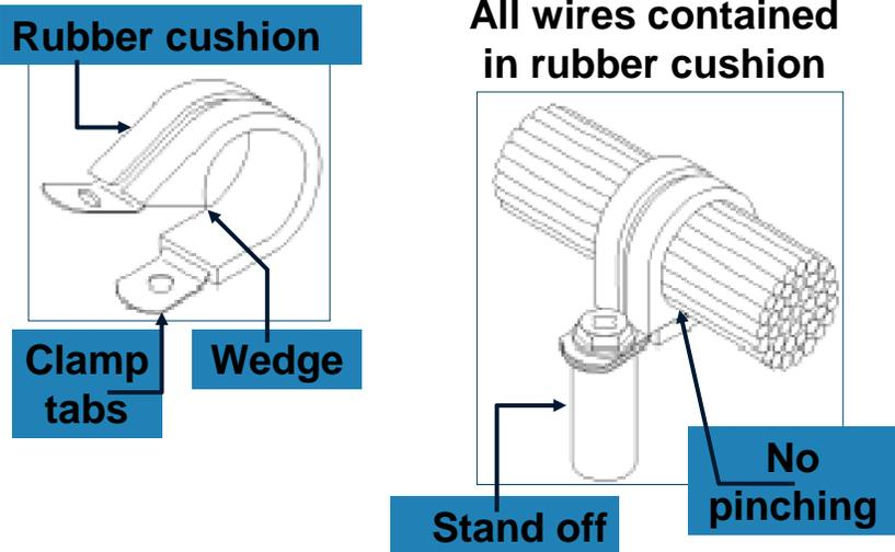
Figure 5. Typical Rubber Clamp (Aircraft Wiring Practices, 2002).
