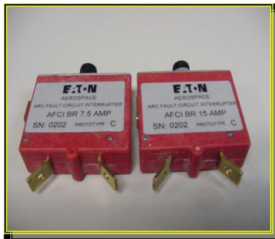
*Figure 19.* Eaton Arc Fault Circuit Breakers (Arnason, 2001).
