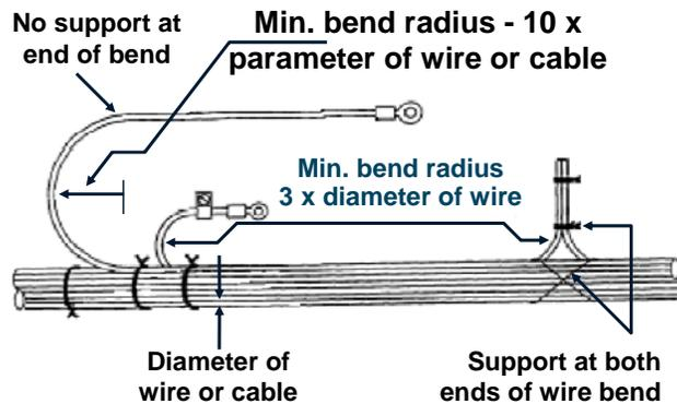
Figure 7. Minimum Bend Radii (Aircraft Wiring Practices, 2002).
