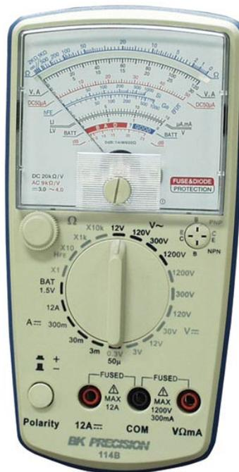
Figure 15. BK114B Analog Multimeter
