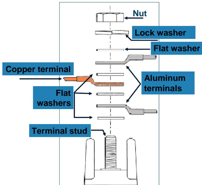
Figure 13. Terminal Stacking Unlike Materials (Aircraft Wiring Practices, 2002).
