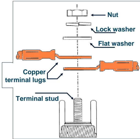
Figure 12. Terminal Stacking Like Materials (Aircraft Wiring Practices, 2002).
