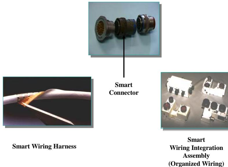
Figure 18. Smart Wiring Technology Subcomponents (Arnason, 2001).
