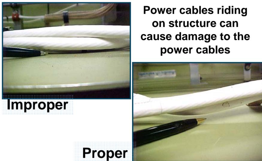
*Figure 3. Wires Riding On Structure (Aircraft Wiring Practices, 2002).*
