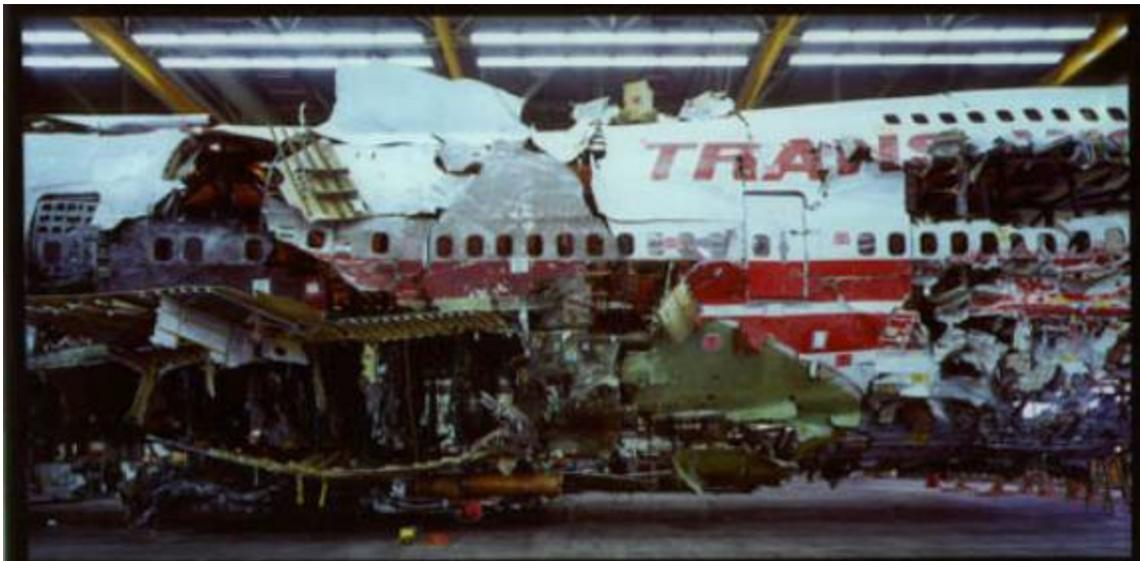
*Figure 1.* TWA Flight 800: The Reconstruction (1999).
