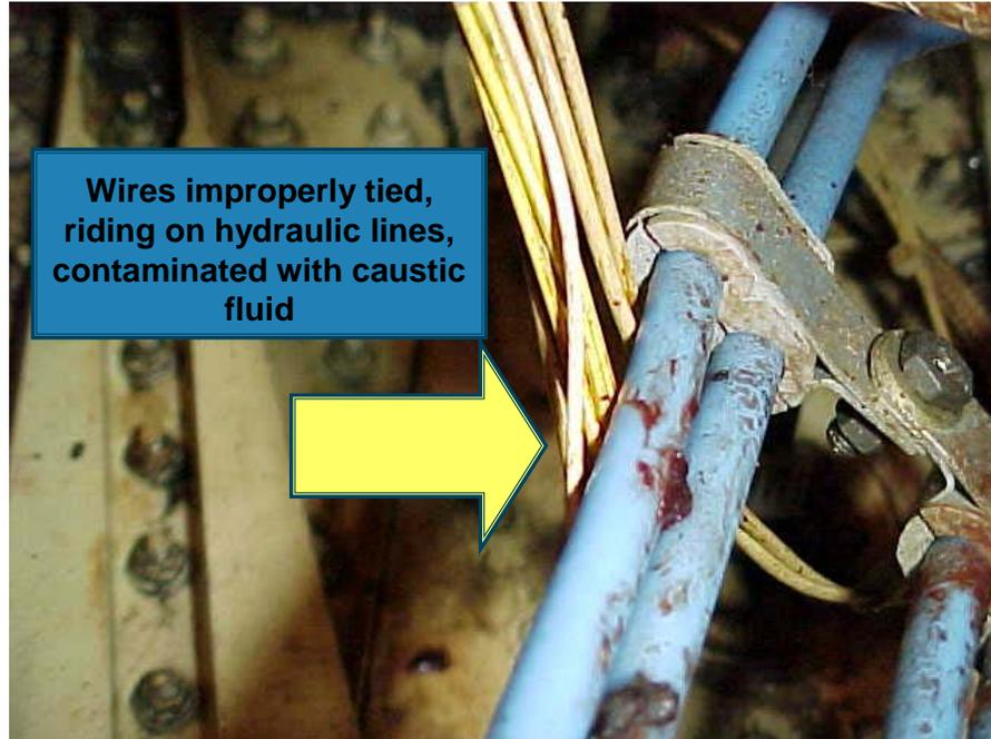
*Figure 4.* Wires Improperly Routed (Aircraft Wiring Practices, 2002).
