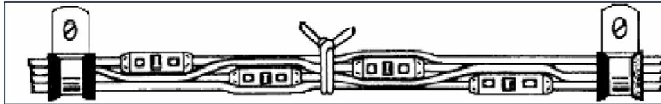
*Figure 11. Staggered Splices (Aircraft Wiring Practices, 2002).*
