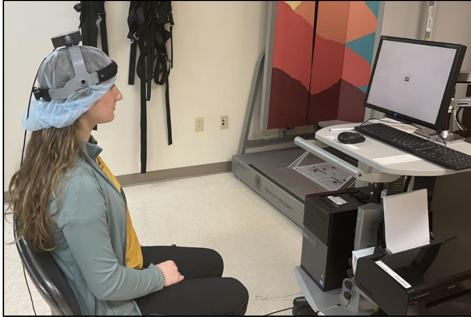
Figure 1. DVA testing using the NeuroCom SMART EquiTest (version 9.2.0) with InVision™ software.
