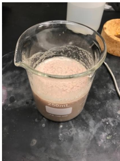
Figure 14: The solid precipitate following the addition of NaOH to the MeOH solution in the synthesis A. This step yields the dipyrin, which should be very active in the visible region.
