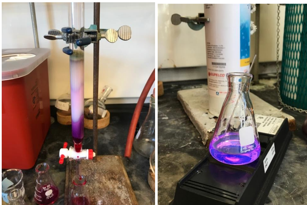
Figure 21: The silica column used to separate the ZnDIPY from the other components of the reaction mixture (left), and the example of a fraction, fraction 10, which was highly UV active (right).
