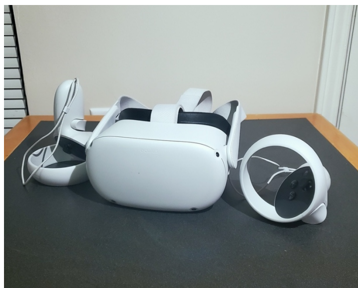
Figure 1. Oculus Quest 2 with its two Oculus Touch Controllers. Both this system and its controllers use 6DOF tracking without the need for any external sensors or wires.
