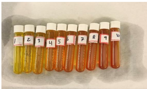
Figure 4. Results of DNS assay with Glucose serial dilution
