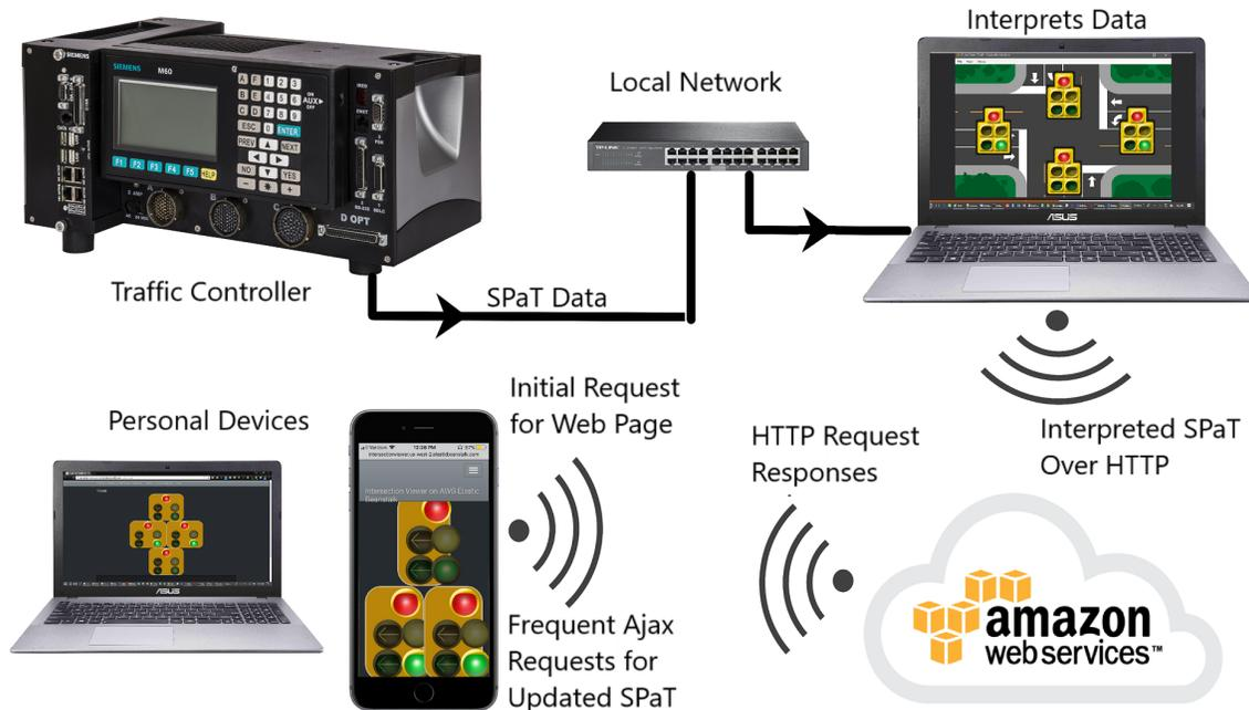
Fig. 1: Overall communication architecture for the application
