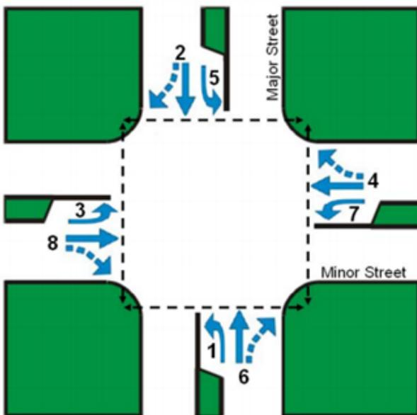
Fig. 2: A standard 8-phase intersection, as used for the application
