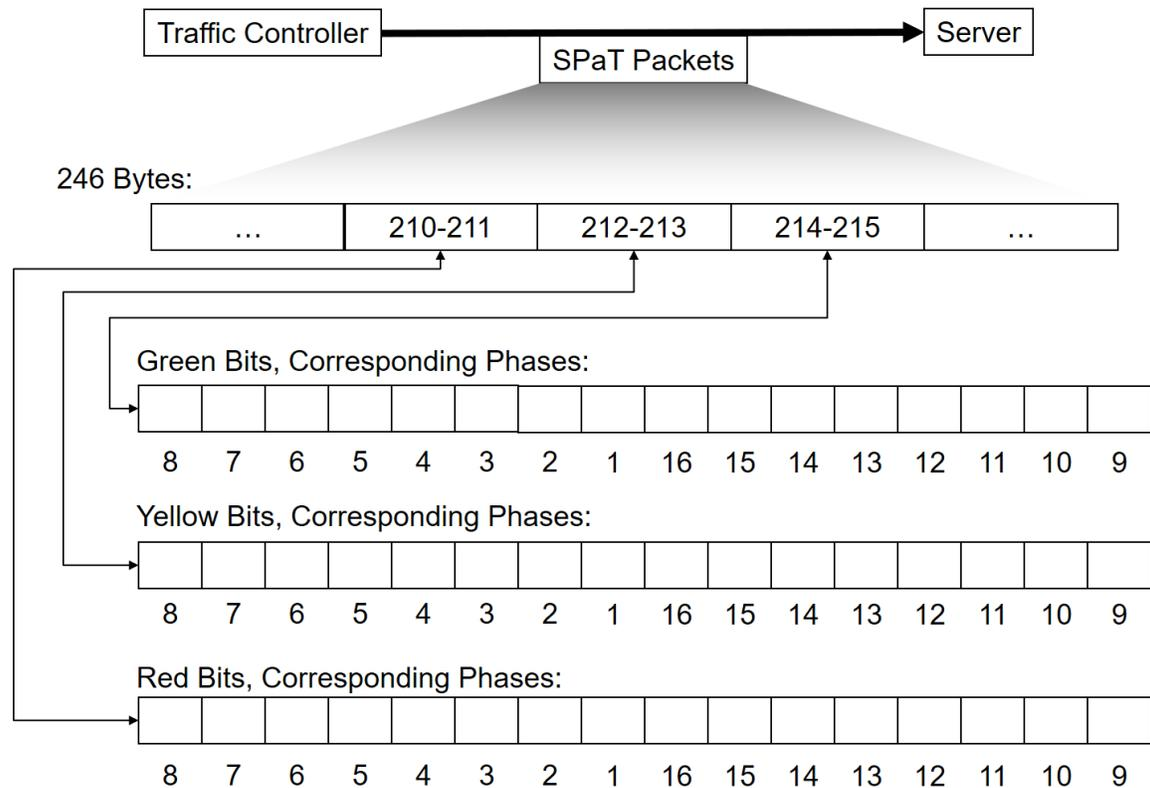
Fig. 3: SPaT packets consist of 245 or 246 bytes. Only certain bytes are relevant for this application.
