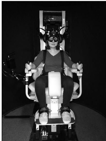
Figure 3. A person secured in the rotary chair, holding two handles with buttons to press for subjective visual vertical (SVV) adjustments. During rotation and SVV trials, the rotary chair booth was completely darkened to eliminate all visual cues other than those provided by the laser target during the experiment.
