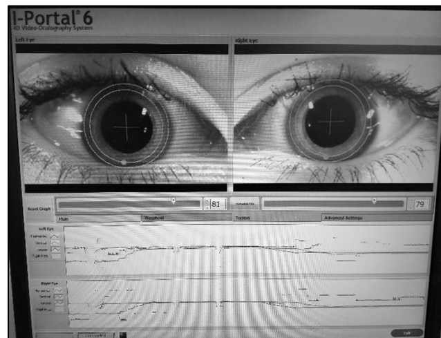
Figure 2. The I-Portal Falcon high speed video-oculography (VOG) system (100 Hz frame rate) for evaluation and recording vertical, horizontal, and torsional eye movements in collaboration with the VEST 8.0.1 operating and analysis software system.
