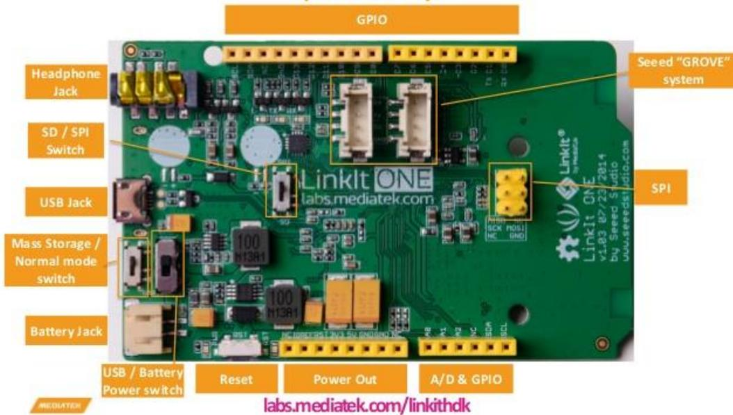
Fig. 3-3 front view: different pins and inputs (MediaTek Labs, 2015)
