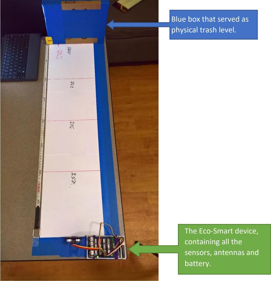
Fig. 9-1: Device testing system.
