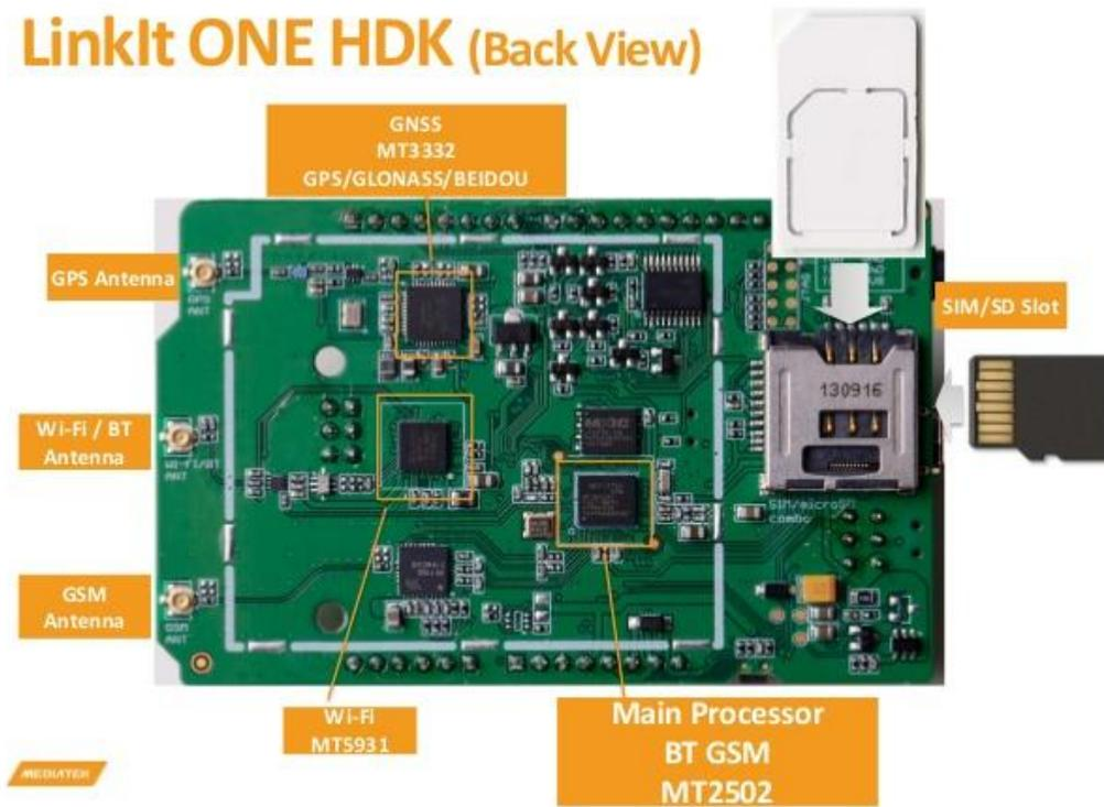
Fig. 3-2: Back view, chips names (MediaTek Labs, 2015)
