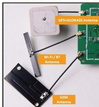
Fig. 3-1: Antenna Ports (MediaTek Labs, 2015)
