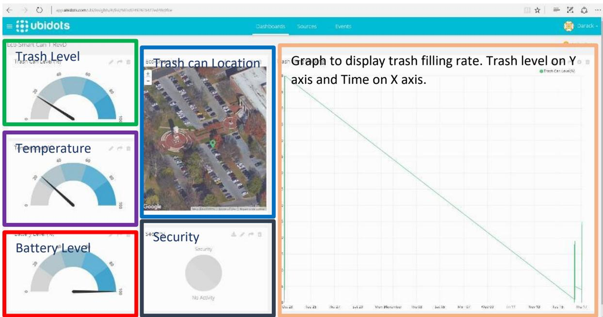
Fig. 9-3: Ubidots cloud service Dashboard
