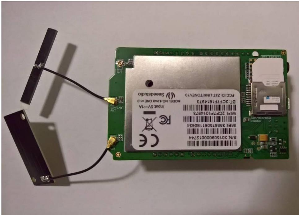
*Fig. 5-1: GPRS & Wi-Fi antenna & Ting 2G Sim card.*
