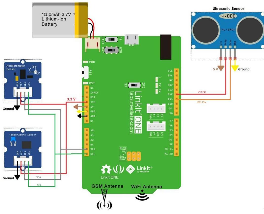
Fig. 4-1: Board connection layout (Developed with Fritzing Software)
