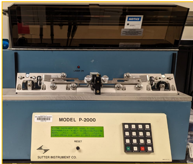
Figure 6. Laser pipette puller used for electrode fabrication.
