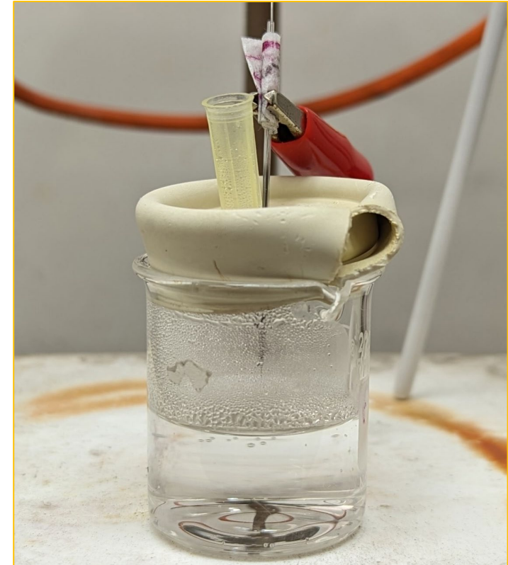
Figure 9. Ammonium hydroxide method of N-doping.
