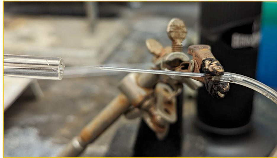
Figure 7. Setup for chemical vapor deposition micro-torch method for making carbon electrodes. Utilizes a 70:30 butane/propane mixture as precursor gas. Opposing argon flow provides inert atmosphere for pyrolysis.
