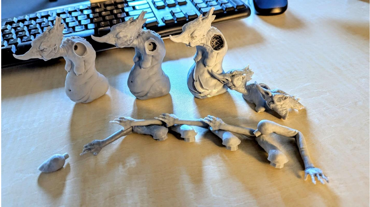
Figure 17. First Set of Failed Prints. You can see the new hexagonal keys for the shoulders, interior supports, as well as the different levels at which the prints were failing.
