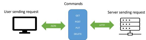
The process of how APIs work consists of an application receiving data and communicating through JSON via an HTTP request in order to get data from a web server.
