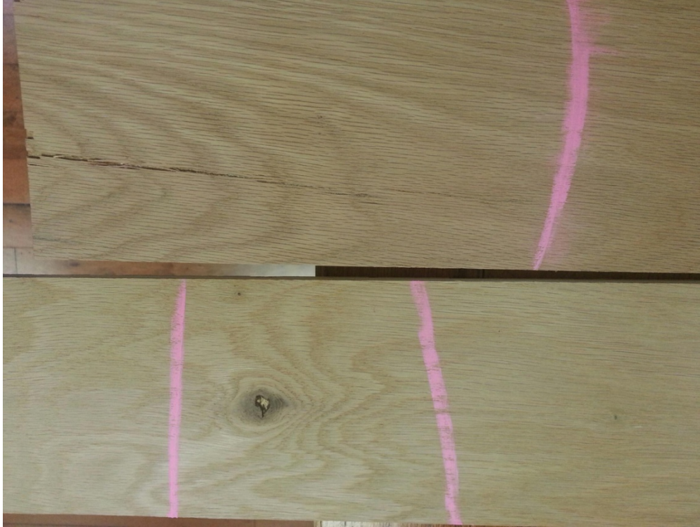
Figure 21: Chalk Mark Location too far Away from the Actual Defect
