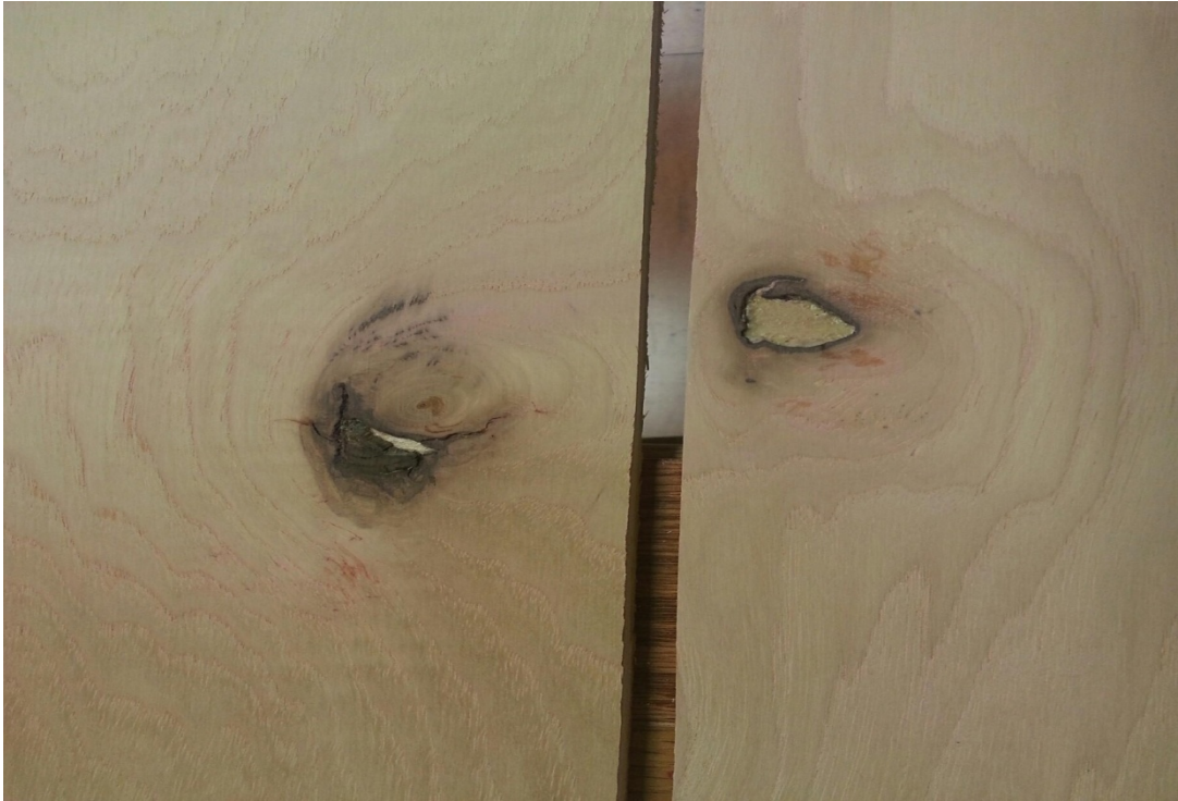
Figure18: Knot Holes in the Face
