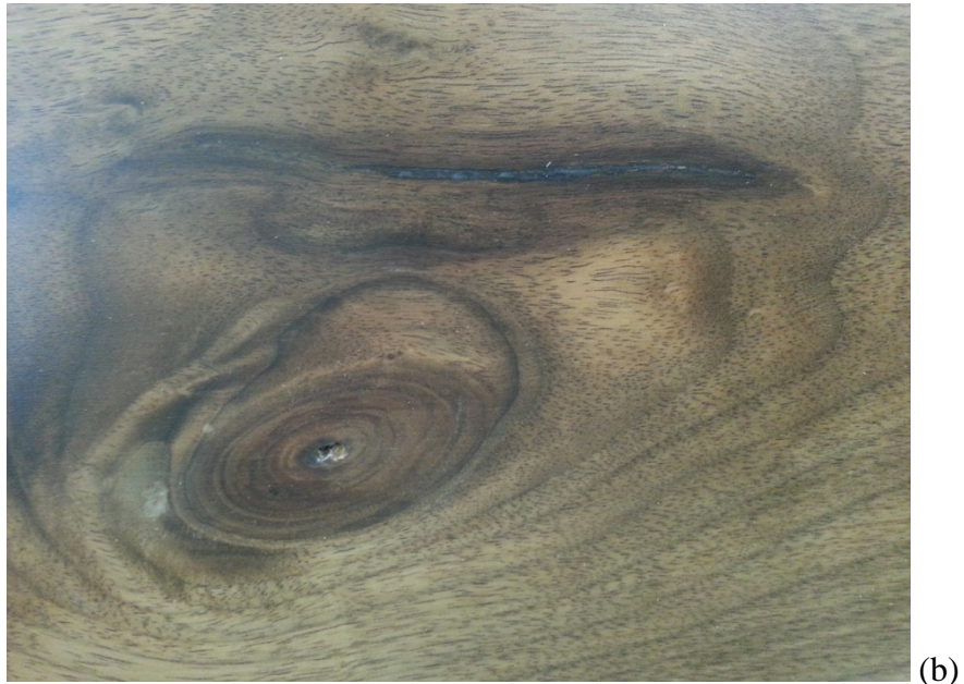
Figure 22: (a) Unfinished Elongated and Circular Defect; (b) Elongated Defect Filled During the Finish Process where as the Circular Defect Did Not Fill
