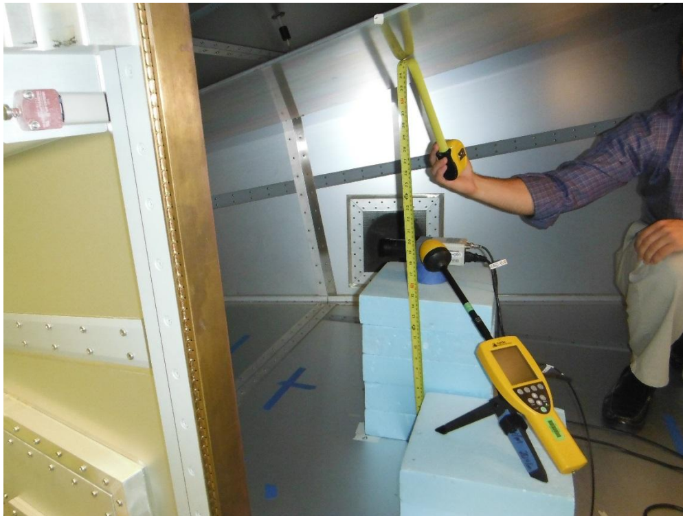
Figure 10: Measuring the Height of the GTEM Septum and Camera
