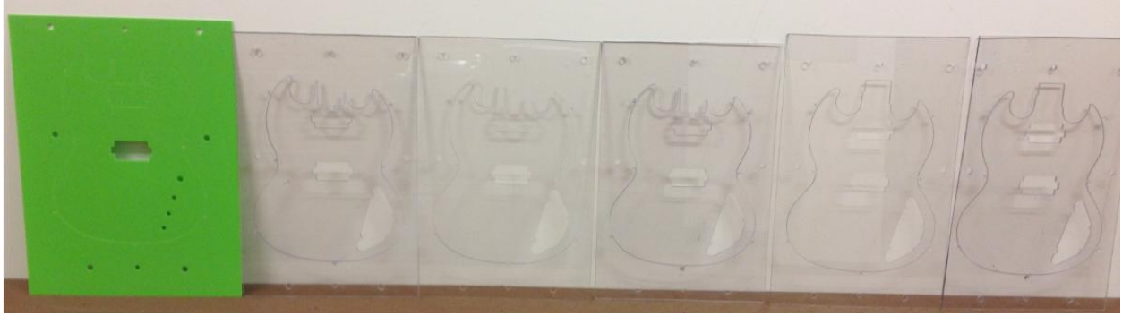
Figure 50. First 6 Layers Cut by the OMAX 5555 JetMachining Center
