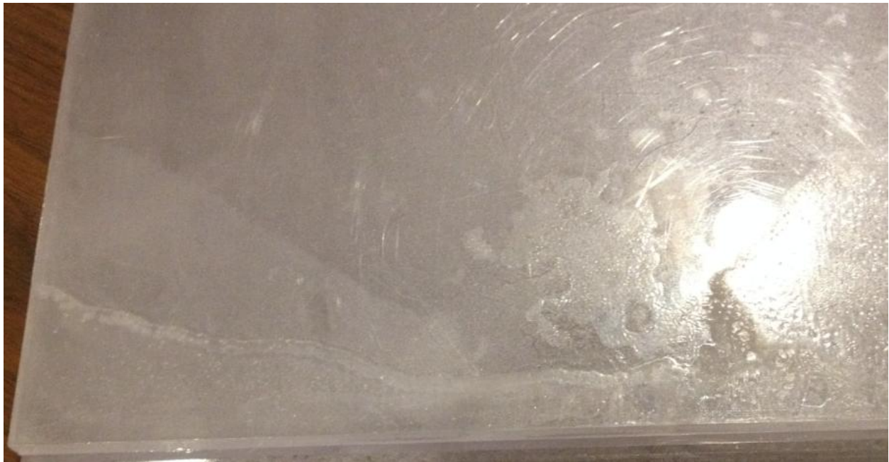
Figure 25. Undesired Solvent Attack
