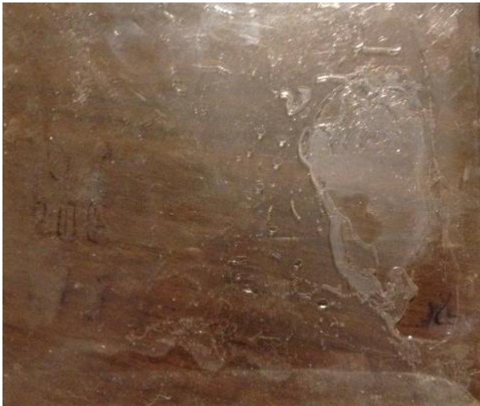
Figure 24. Example of MEK Laking
