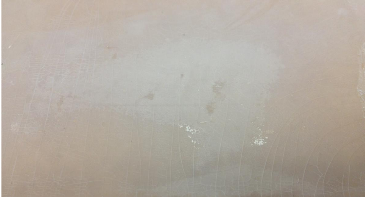
Figure 22. Example of Stress Fracturing Induced by Application of Acetone
