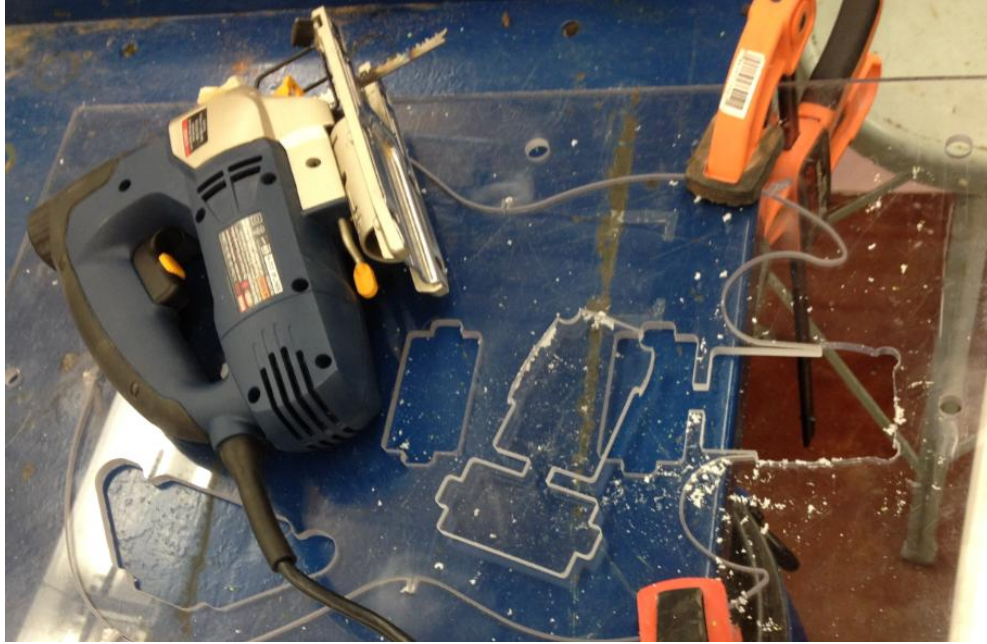
Figure 56. Jigsaw Removal of Neck Pocket Geometry
