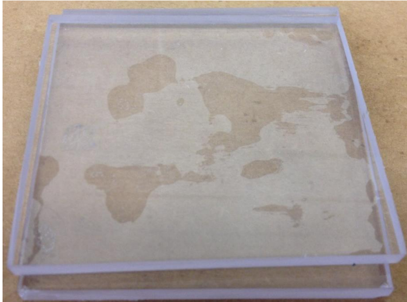
Figure 33. Liquid Methylene Chloride Test Specimen Exhibiting Laking
