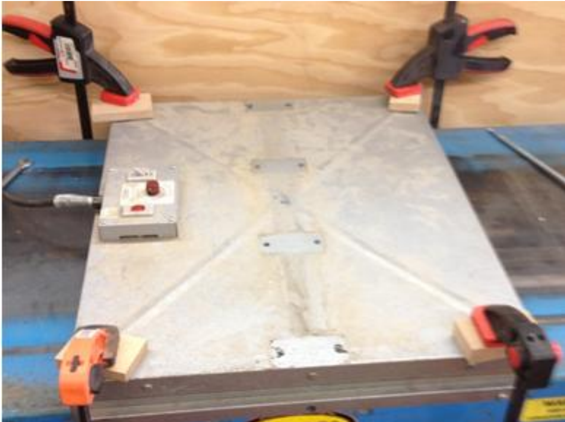
Figure 19. Clamps Applying Vertical Compressive Force to 16" x 12" Test Specimens
