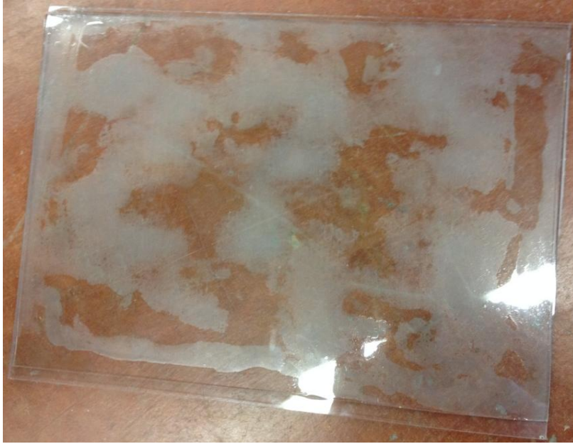
Figure 20. Resulting Air Pockets in the 16" x 12" Test Specimens (30 Minutes at 180°F)
