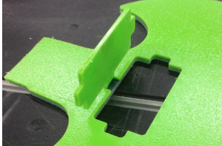
Figure 54. Example of Undesired Neck Pocket Bonding
