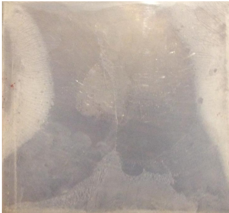
Figure 21. Example of Hazing and Crystallization with Acetone
