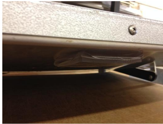
Figure 15. Test Squares Fused to Heat Plate (30 Minutes at 250°F)
