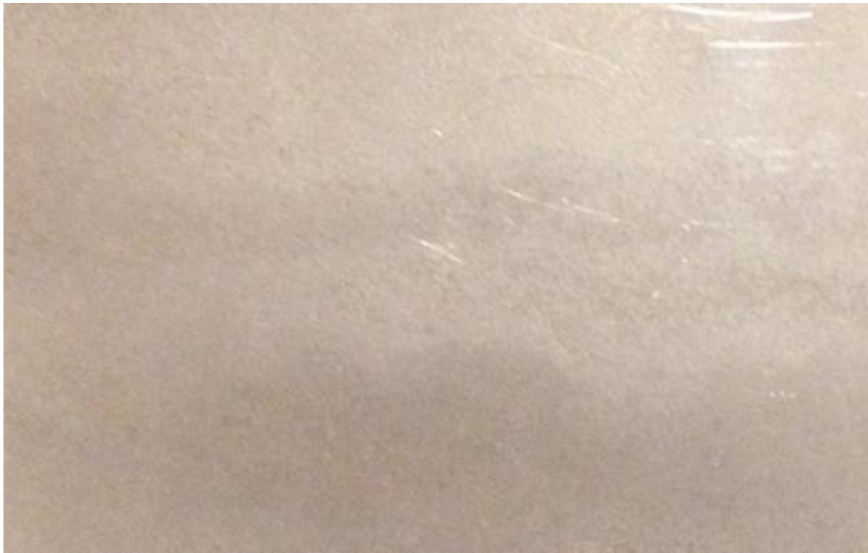
Figure 35. Uniform Frosted Bond Appearance of Loctite® Spray Adhesive Test
