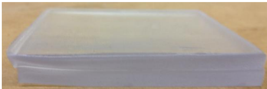
Figure 18. Deformation Due to Angular Compression of Technal Model 550 Dry Mount Press
