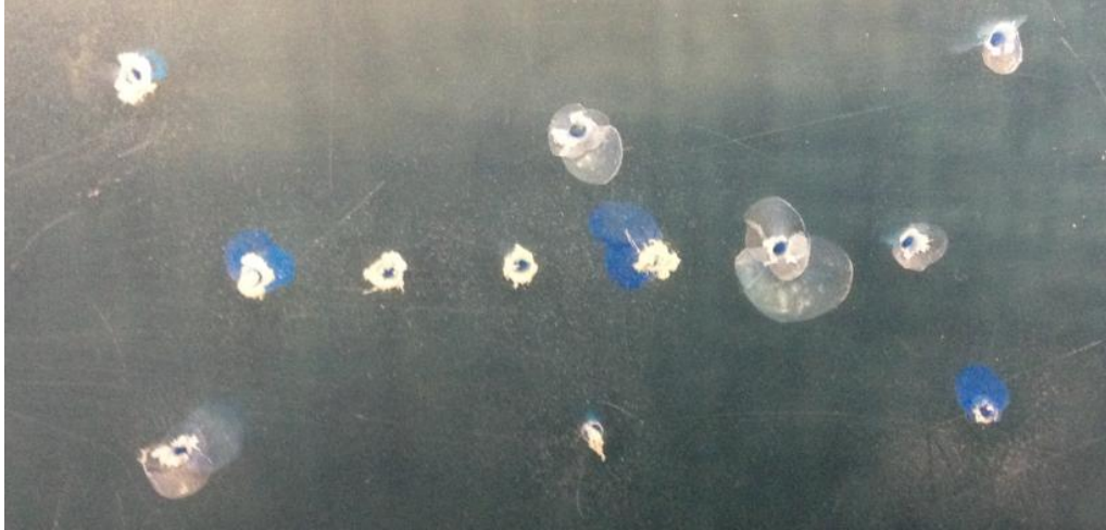
Figure 45. Example of Blowout in 4mm Copolyester
