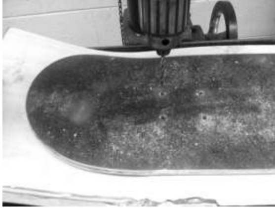
Figure 28. Drilling Operation Using Master Deck as Template
