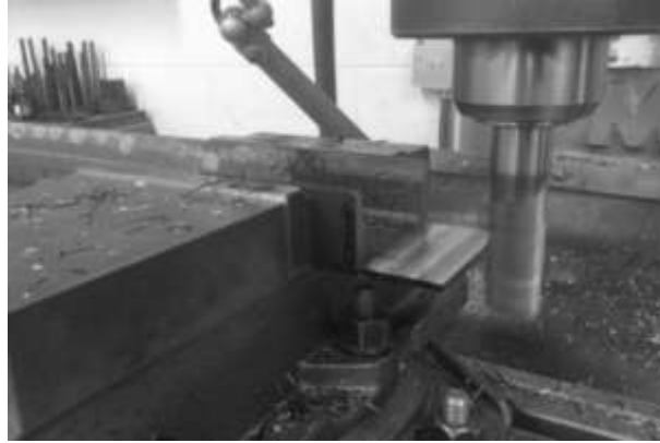
Figure 12. C-Channel Being Milled to Final Length with Recess Being Milled into Surface
