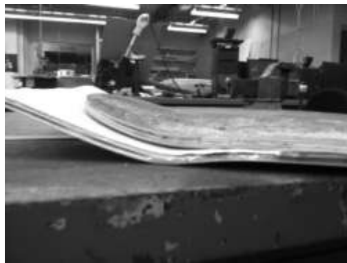
Figure 26. Master Deck Being Mounted and Indicated on Blank Deck
