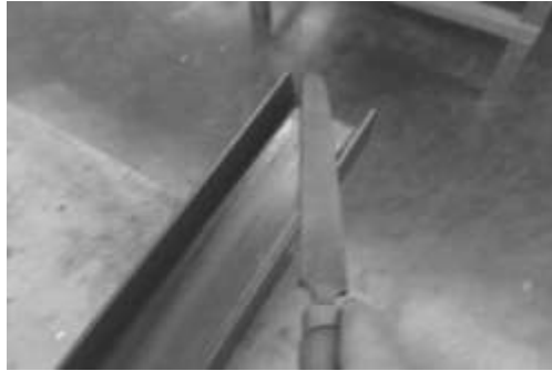
Figure 14. C-Channel being De-burred after Cutting and Drilling Operations
