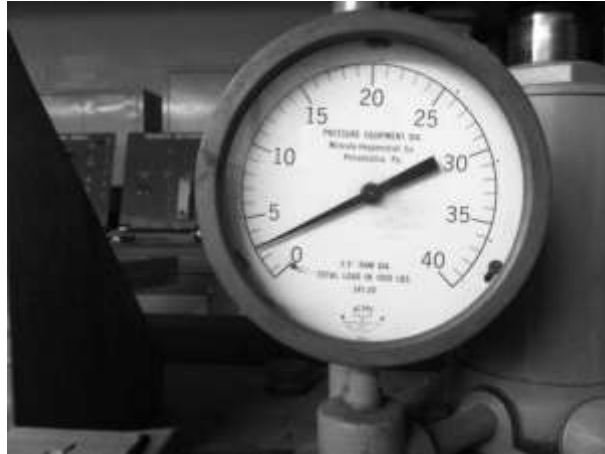
Figure 40. Deck Tongue Rating Reading Nearly 3,000 Pounds Prior to Failure
