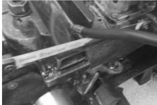
Figure 11. C-Channel Being Cut to Length Using Reciprocating Saw
