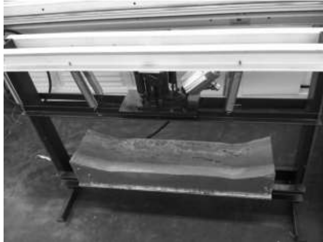
Figure 17. Drag Mold Mounted to Frame, and Springs Loaded in Respective Positions
