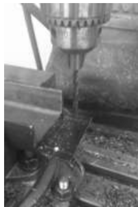
Figure 13. C-Channel receiving 3/8" Drill Holes after being Center Drilled.
