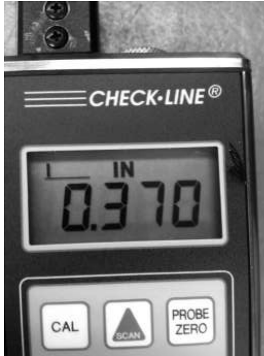
Figure 41. Ultrasonic Thickness Tester Reading at Nominal Thickness
