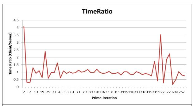
Figure 3: Graph of Client/Server computational time ratio per iteration,  $TimeRatio_n$ . After some preliminary imbalance, the load balancer reaches approximate equilibrium. Concurrent calculation ends as the time ratios become more chaotic.
