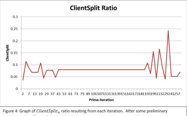
Figure 4: Graph of  $ClientSplit_n$  ratio resulting from each iteration. After some preliminary imbalance, the effects of the threshold-based approach can be seen, translating approximate  $TimeRatio_n$  equilibrium into a steady  $ClientSplit_n \approx 0.08$ . Concurrent calculation ends as  $ClientSplit_n$  becomes more chaotic.
