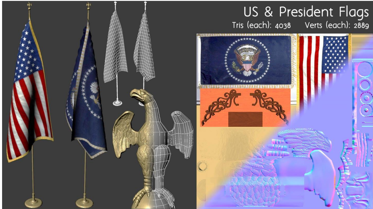
Figure 13: The final flags with the model's wireframe (left) and the Diffuse and Normal maps (right).
